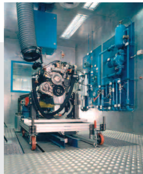
Motorprüfstand in Containerbauweise Engine test stand as container construction
